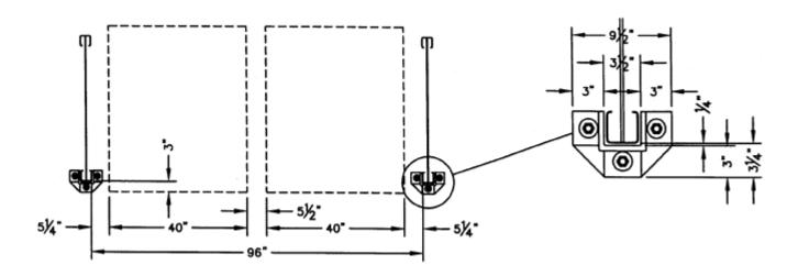
Defender Foot provides indestructible protection for rack columns. This ductile iron casting column protector eliminates damage even when subjected to repeated impact abuse by reach truck straddles.
